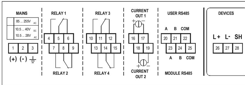
After loosening threads and removing cover of the wiring terminal the cables can be connected. The same cable should not be used for AC and DC as well as different cables should be applied for SELV and mains voltage.
