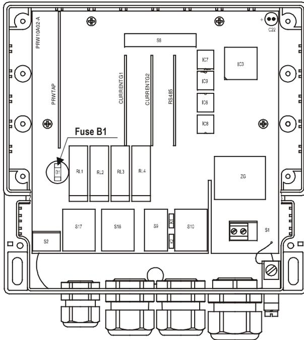
Loosen four nuts, which are fastening the front panel. Tilt forward the front panel carefully, in order not to span cable band and replace the fuse.
