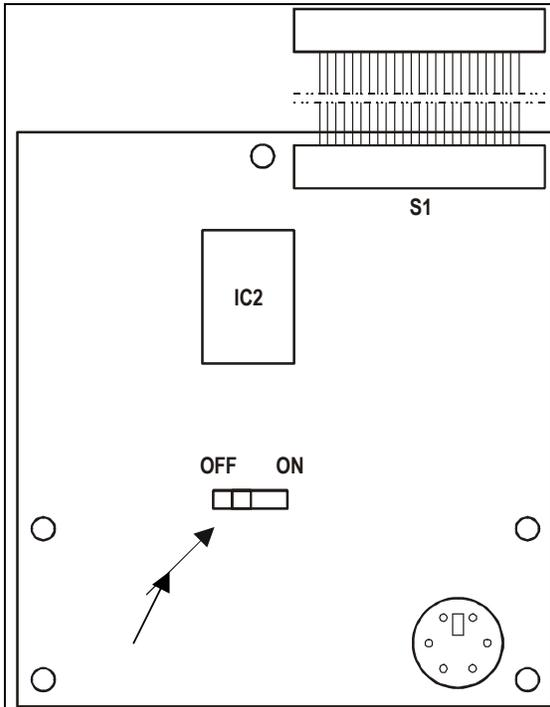
Protection switch can be accessed after loosening nuts fastening the front panel.
